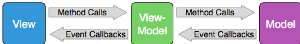
MVVM was designed to take advantage of XAML and particularly XAML-based data bindings. Generally, the View is a page class that uses XAML to construct the user interface. Therefore, the connection between the View and the ViewModel consists largely—and perhaps exclusively—of XAML-based data bindings:
